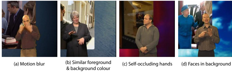
Fig. 3. Challenges in the BBC TV Signing dataset. (a) Motion blur removes much of the edges of the hand; (b) similar foreground & background colours render colour information less informative; (c) self-occluding hands makes the assignment of left/right hand ambiguous; (d) faces in the background renders face detection-based bounding box detection difficult.
