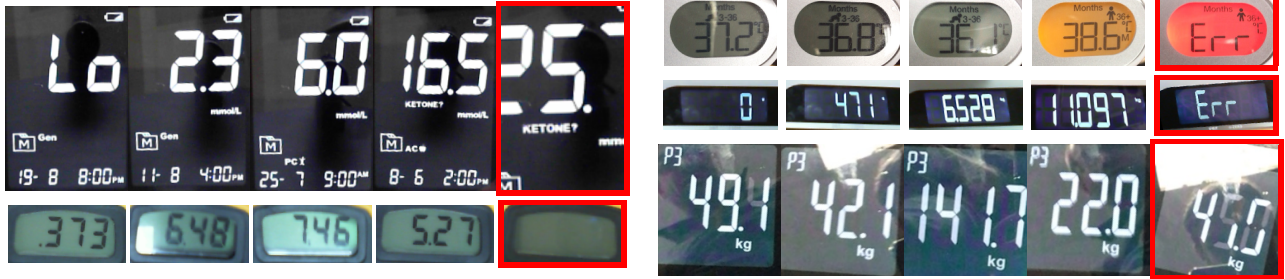
Figure 5. Digit-recognition dataset. 5 example screen snapshots from each of our digital meters is shown. First four columns are valid examples with the last column an invalid example (marked with red border). Notice the difficulty in recognizing the digits due to lighting and reflections.
