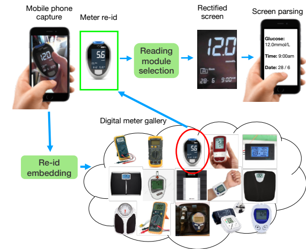
Figure 1. Recognition and screen reading on mobile phone. Our system can both recognise and parse the screen of a digital meter at near 100% read accuracy. The system is trainable using a single human labelled image consisting of a binary mask indicating screen and background pixels, and the four corner coordinates of the screen, see Figure 2. For meter recognition the system matches a deep re-id embedding to the best matching meter in a gallery of collected digital meters.
